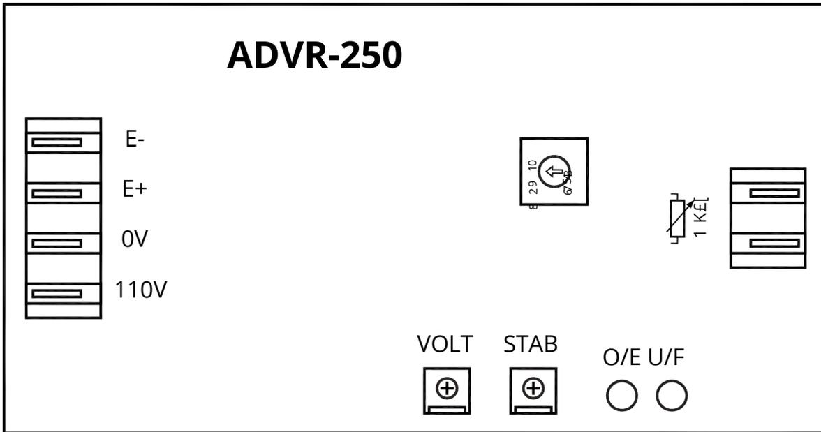
**0V 110V : Power Supply and Sensing Input**
